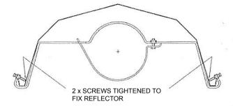
Type 'S' are sliding reflector brackets.
