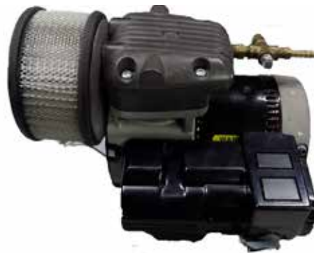
Figure 4. Replacement Compressor with Air Manifold and Air Filter Assemblies Installed
