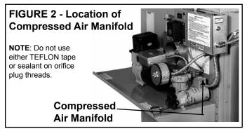
Unscrew the orifice and discard. Install the #70 orifice furnished in the option package.
